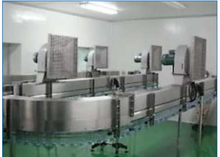
EMPTY BOTTLE AIR CONVEYOR SYSTEM WITH AIR BLOWER AND FILTER
